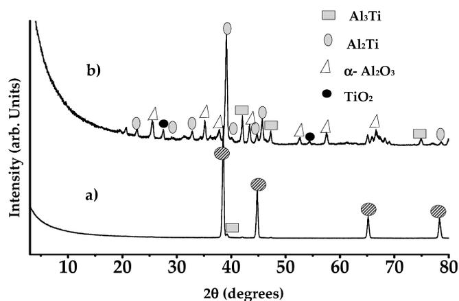
**Figure 5.** TF-XRD of Al layer on the Ti alloy after heat treatment at 640 °C for 12 h (a) and subsequent heat treatment at 850 °C for 96 h (b) both in an air atmosphere. Reproduced from [100] with permission from Trans Tech.
