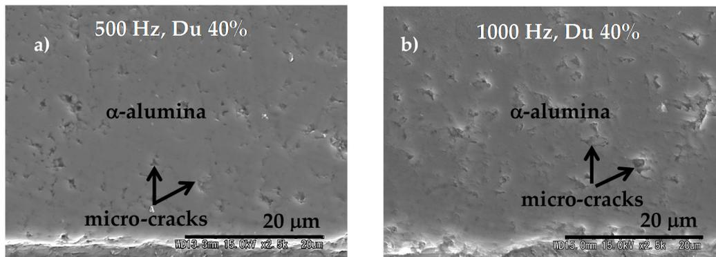
**Figure 8.** SEM image of cross-section of alumina layer on the Ti alloy formed by MAO of CS-Al layer at pulse frequency of 500 Hz (a) and 1000 Hz (b) both at duty cycle of 40% for 60 min. Reproduced from [102] with permission from Elsevier.
