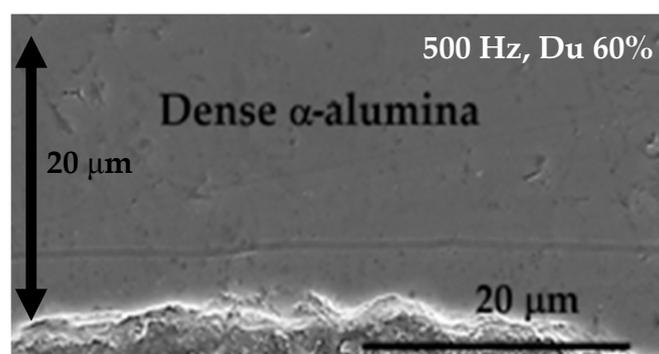
**Figure 9.** SEM image of cross-section of alumina layer on the Ti alloy formed by MAO of CS-Al layer at pulse frequency of 500 Hz and at duty cycle of 60% for 60 min. Reproduced from [102] with permission from [102].
