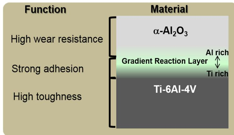
**Figure 12.** Schematic of cross-sectional view of a  $\alpha$ -alumina layer on the Ti alloy with a gradient reaction layer at their interface. Reproduced from [103] with permission from Cambridge Core.
