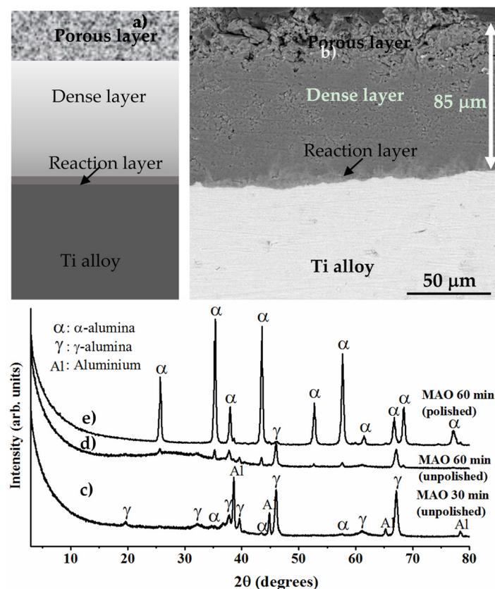
**Figure 7.** Schematic view of section of designed alumina/Ti alloy model (a); corresponding BSE image of alumina layer on the Ti alloy (b); and TF-XRDs of CS-Al layer after MAO for 30 min (c); 60 min (d); and after polishing (e). Reproduced from [101] with permission from Elsevier.
