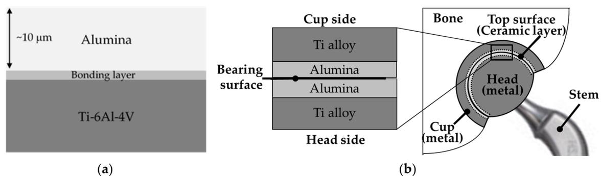
**Figure 1.** Cross-sectional views of alumina/Ti alloy (ATH) hybrid model (a), and ATH-on-ATH configuration of the artificial hip joint (b). Reproduced from [102] with permission from Elsevier.
