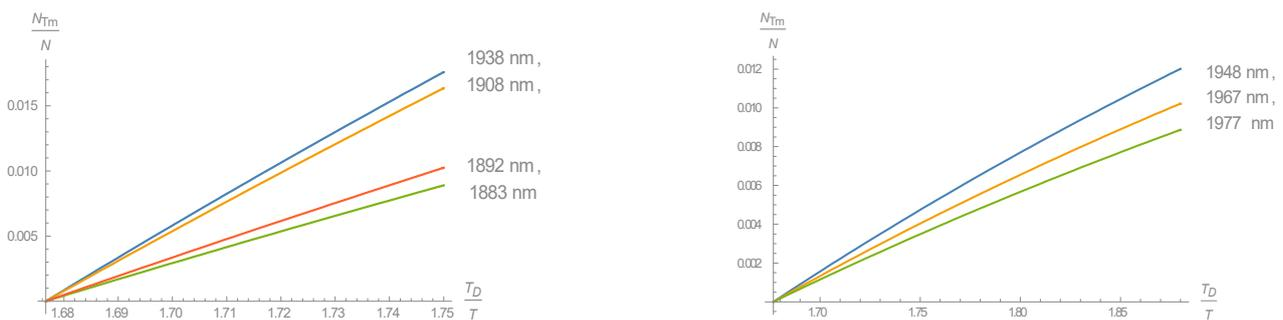
**Figure 3.** Concentration dependences of the cooling temperature at the excitation intensity  $F_p = 5 \times 10^{21} \text{ cm}^{-2}\text{s}^{-1}$  at wavelengths leading to the most efficient cooling.
