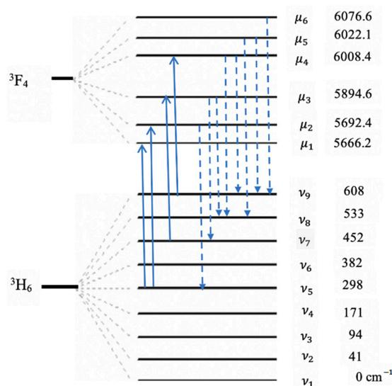
Figure 1. Energy levels scheme of <sup>3</sup>H<sub>6</sub> and <sup>3</sup>F<sub>4</sub> manifolds Tm<sup>3+</sup> ion in LN [9].
