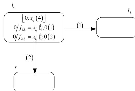
Figure 8. The deterministic ADD module in system  $\Pi_2$ .
