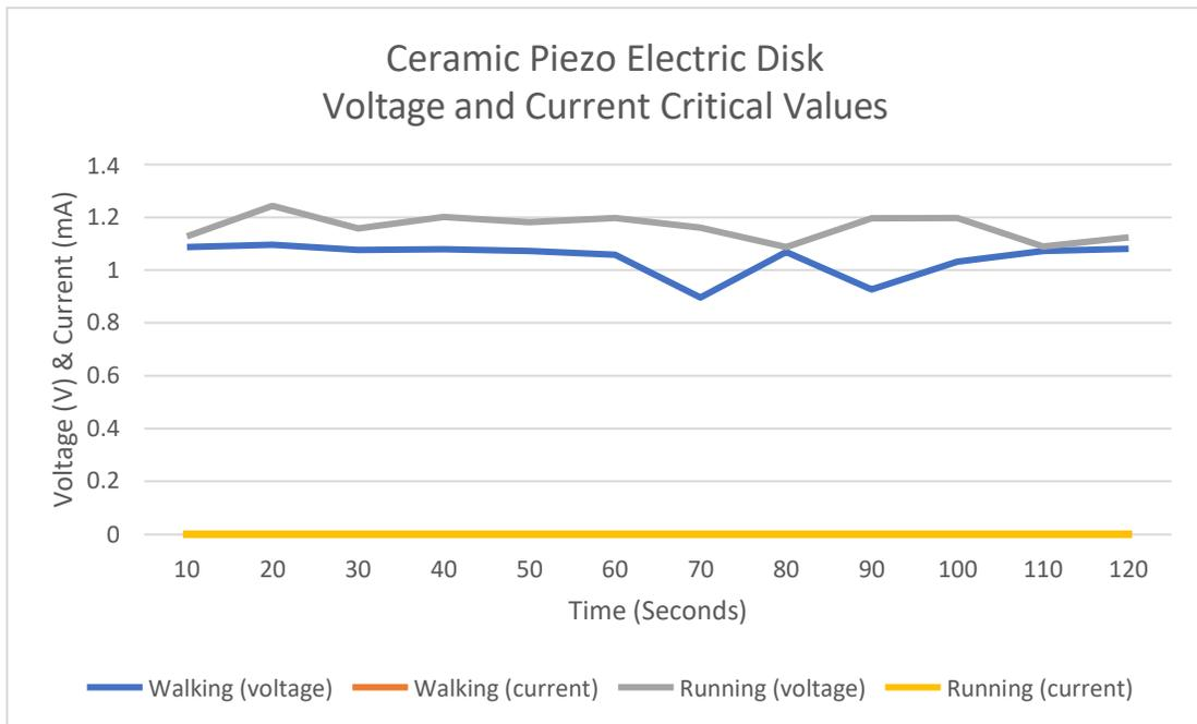
Figure 7. Critical Values of Piezoelectric disk
