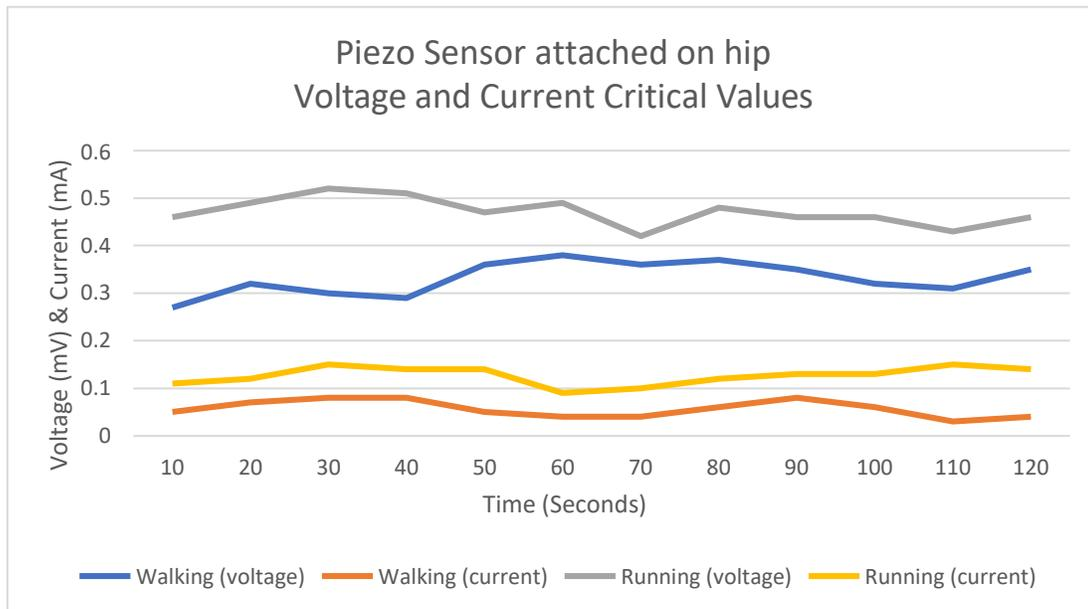
Figure 9. Critical Values of Piezoelectric strip attached to hip
