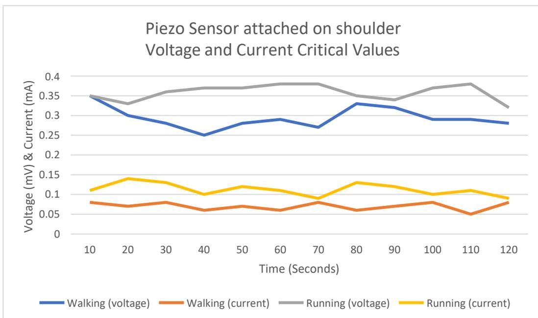
Figure 8. Critical Values of Piezoelectric strip attached on shoulder
