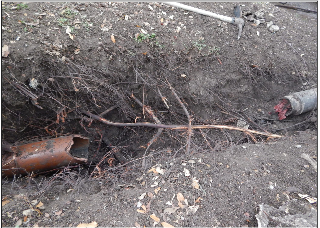
Figure 4-4. Trench profile at end of excavation. Note broken pipe, extensive roots, and silty deposits.
