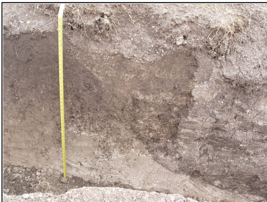
Figure 4-9. Close-up of the edge of the acequia trench showing the contrast between mottled matrix on the inside of the trench and dark gray matrix on the outside (left of photo).
