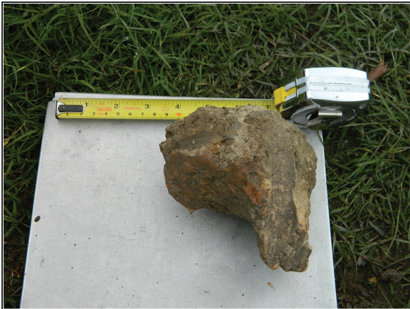
Figure 4-11. Fragment of burnt daub showing vertical pole (semi-circle at front) and perpendicular stick impressions indicative of a corner segment.
