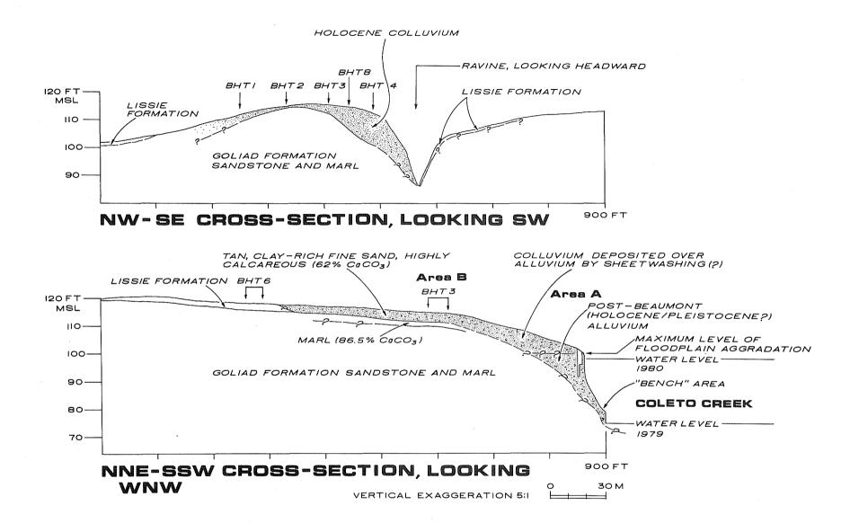
Figure 5. Cross Sections of Geologic Units at the Berger Bluff Site (41 GD 30), Based on Backhoe Trenching and Hand Excavation. The lower section is somewhat similar to Figure 3 in Brown (1983) but is based on much more data and is therefore more accurate. Elevations represent feet above mean sea level. The 1979 excavation block is shown near the edge of the bluff. Note vertical exaggeration.
