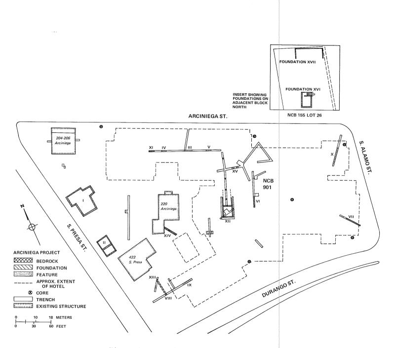
Figure 4. Location of Excavated Foundations.
