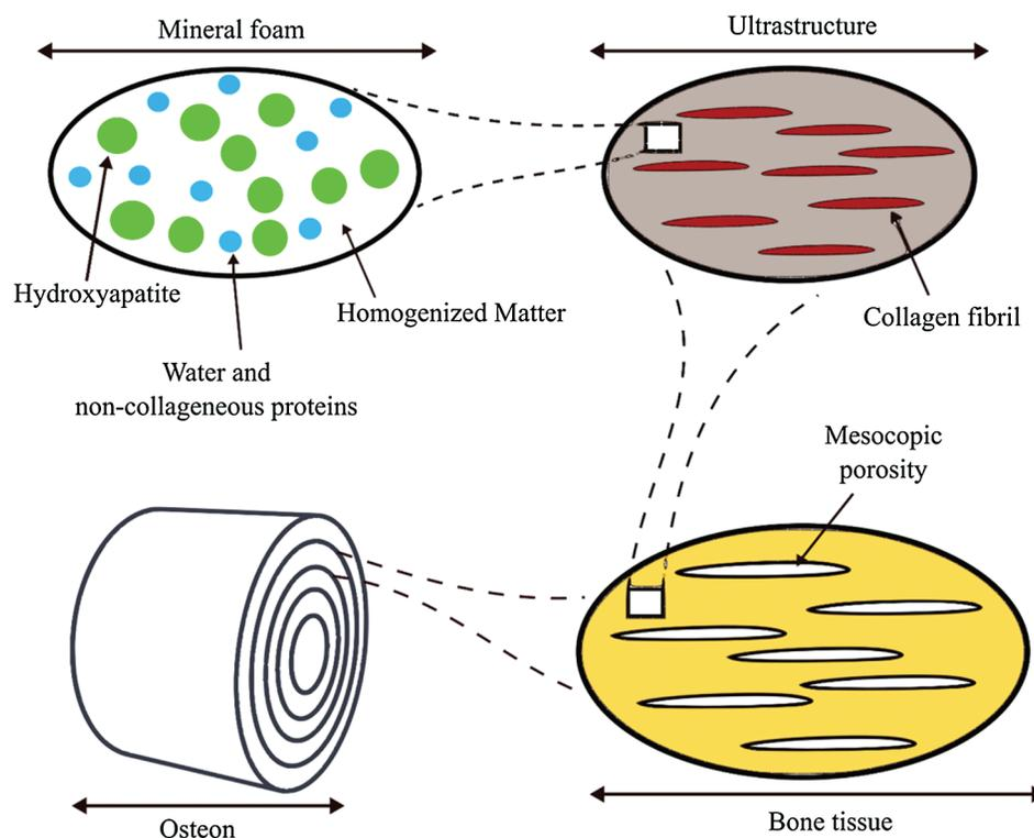
**Figure 6:** Multiscale micromechanical models considering bone as mineral foams reinforced by mineralized collagen fibrils [194]
