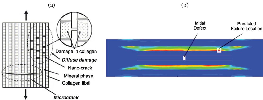
**Figure 5:** Probabilistic models based on simple geometries: (a) a two-dimensional shear-lag based model built to analyze the damage mode, microcrack progression and stress concentration in neighboring mineral phases [191], (b) studying the effect of mineral–collagen interface on the damage mode and microdamage progression [189,190]
