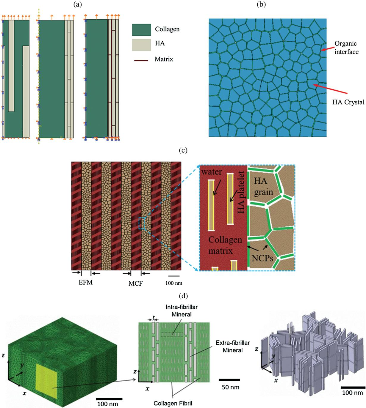
**Figure 4:** FE modeling of sub-lamellar bone: (a) the effect of placing mineral phase inside or outside of the fibrils was studied in [71], (b) bone extrafibrillar matrix was considered as a nanocomposite of mineral crystals bound together by thin layers of relatively soft non-collagenous proteins [151], (c) two-dimensional [187] and (d) three-dimensional models accounting for more detail composition of mineralized collagen fibrils and extrafibrillar matrix [149]
