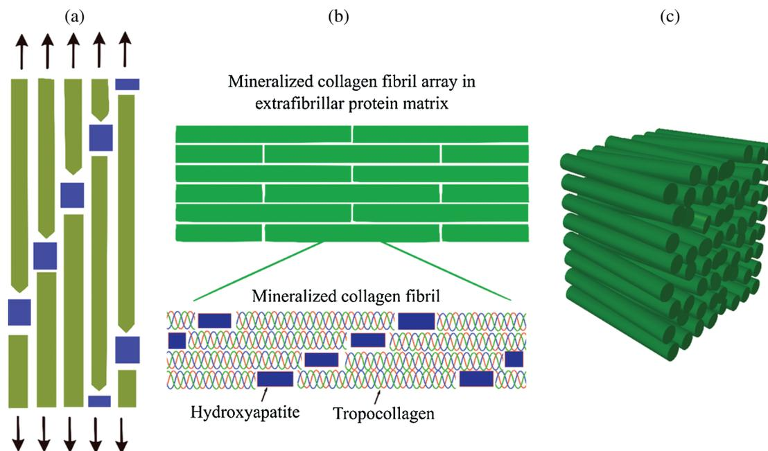
**Figure 3:** FE modeling of mineralized collagen fibrils: (a) a two-dimensional study considering the effect of cross-links [161], (b) a two-dimensional study considering an array of mineralized collagen fibrils [180], (c) a model investigating a three-dimensional network of mineralized collagen fibrils [181]
