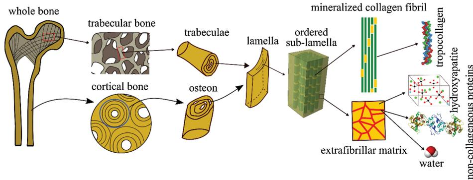
**Figure 1:** Schematic representation of hierarchical structure of bone spanning from whole organ to the nanoscale ingredients
