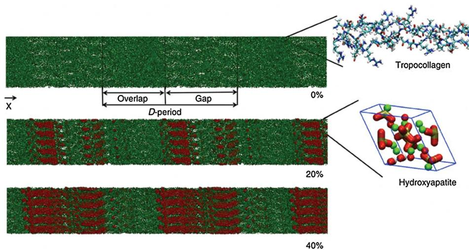
**Figure 7:** Molecular dynamics studies of bone using full-atomistic three dimensional study of mineralized collagen fibrils with different degrees of mineralization [198]
