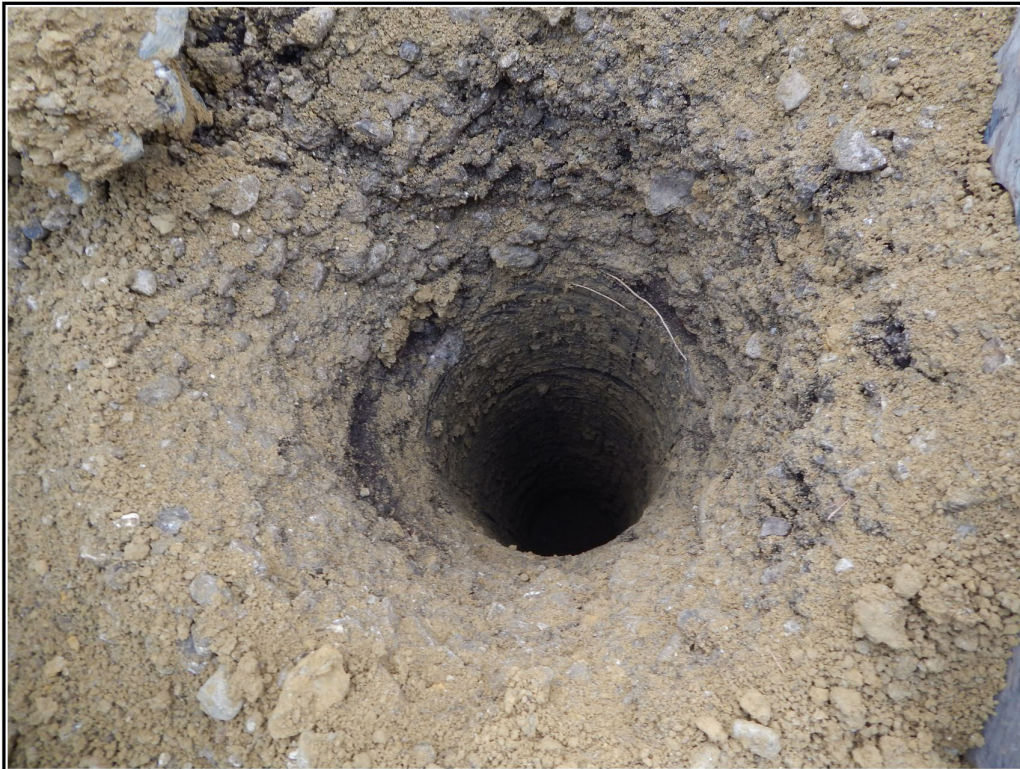
Figure 4-2. Pole hole excavated at 1212 Perez. Note clumpy clays near the surface, sand deposits near the bottom.
