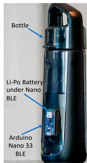
**Figure 1.** Instrumented bottle setup.
