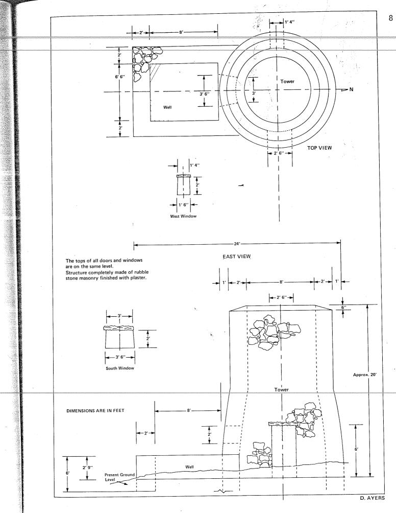
Figure 5 Details of Well Tower Constituetion
