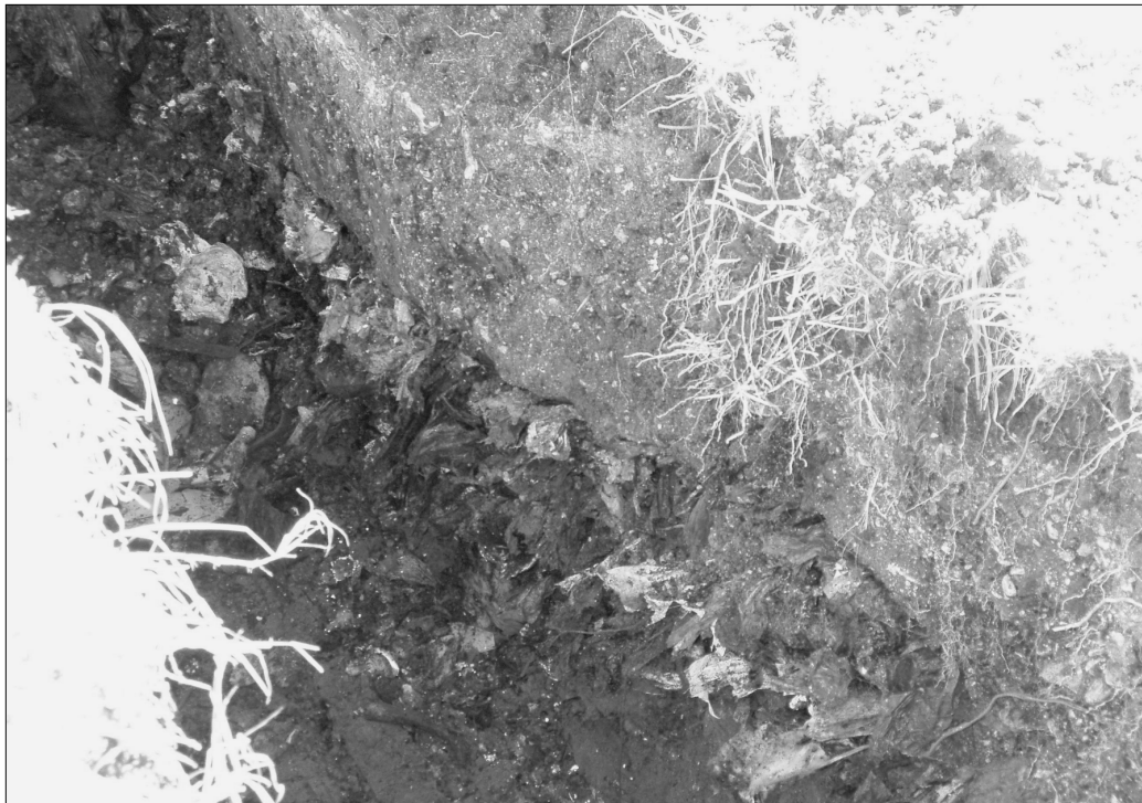
Figure 4-4. Landfill material encountered in Backhoe Trench 2.
