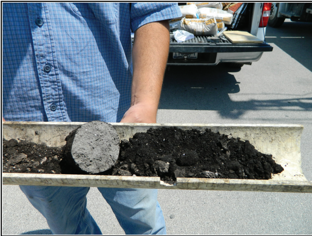
Figure 4-2. Light gray Navaro Clay formation overlying the charcoal layer that is 66-cm thick in this core extracted from the western half of the property.
