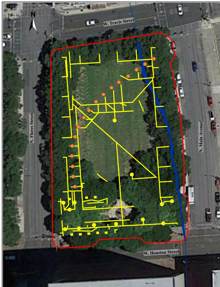
Figure 4-1. Google Earth image of the project area (red outline) showing a series of piers for light fixtures and utilities to be installed across the site (yellow outlines), including 17 piers for a planned pergola (orange dots). Note georeferenced trace of the San Pedro Acequia (blue outline).
