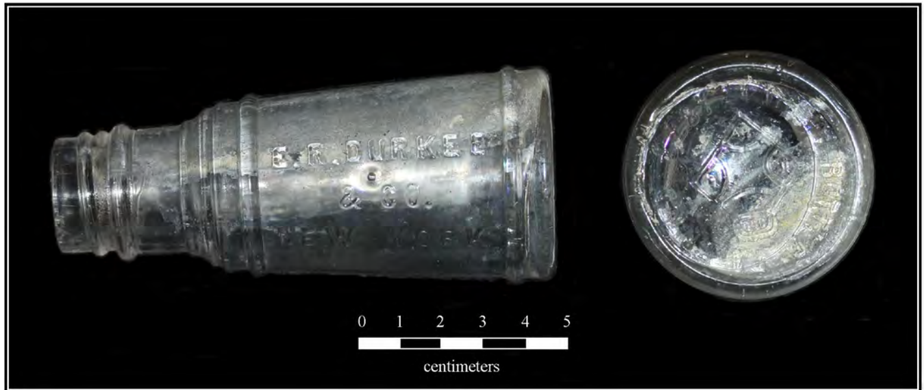
Figure 4-4. Durkee salad dressing bottle and base; note Owens machine suction scar.
