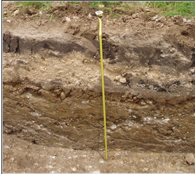
Figure 3-5. East wall of the south half of Trench 3, showing layers of fill to 1.8 m below surface.
