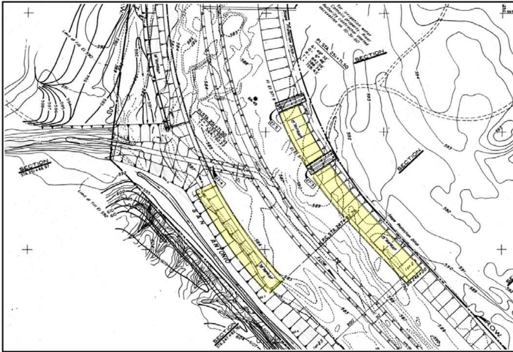
Figure 3-13. Detail plan for Area 3, from original plans for rechannelization of the river. Note reference to riprap along embankment walls (U.S. Army Corps of Engineers, Ft. Worth District, San Antonio River Channel Improvements Detail Plan, Sheet 27.2, 1957).
