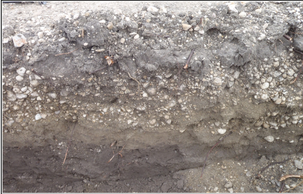
Figure 3-14. South wall of Trench 6 in Area 3. Note gray clay layer at bottom of trench.
