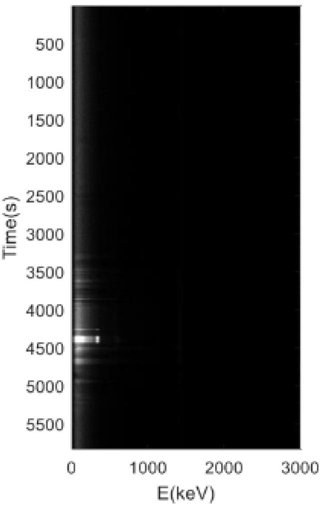
• The white in the grayscale image represents the anomaly signals and the black is background data. Sample from this image were used to create the 3SAT problem, and Grover's algorithm is used to search for the solutions.
