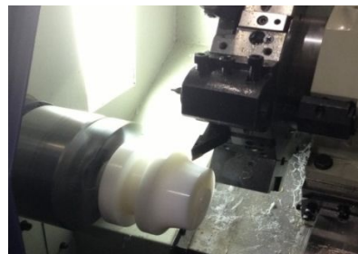
(b) Perform turning for shroud surface (impeller stock)
