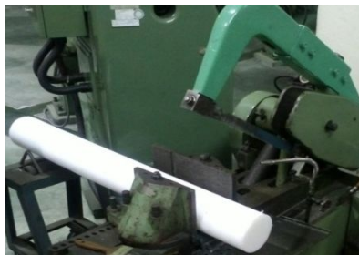
(a) Cut the cylinder bar to impeller height
