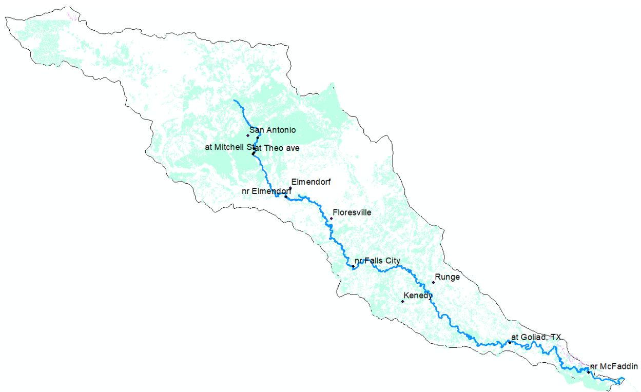
Figure 2.4: Vertisols soil map of San Antonio River watershed. Floresville (08183200), Kenedy (08188060) and Goliad (08188500). Area of vertisols shown by green color.
